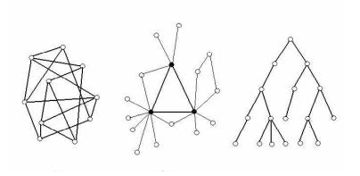
Three types of control structures. Type (a) represents a network; (b) is a hybrid structure while type (c) depicts a hierarchical control structure.
